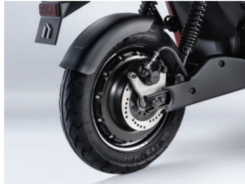
Dual disc brakes for better braking power
